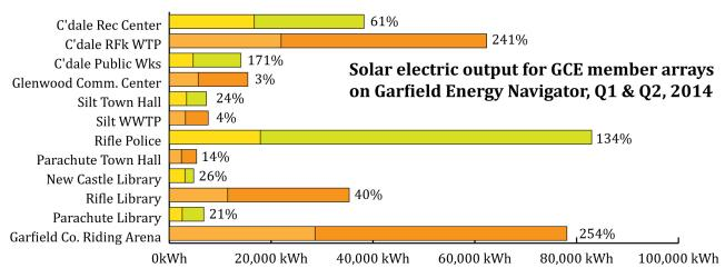
**Notes**: (1) Percentage figures are the Q2 averages for percent of total building electrical energy use offset by solar PV. (2) City of Rifle Wastewater Treatment Plant solar array is not shown here because it is off the charts, producing 1.6 million kWh in Q1 and Q2 combined, which is 161% of the facility's usage.
